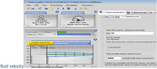
2. We just then entering a speed of movement, almost zero (0.01 msec: zero fluid velocity is forbidden in the calculations, it is necessary to enter a value close to zero to simulate a zero speed).
